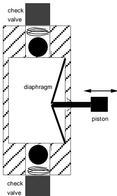
**Figure 3 - Diaphragm Pump**
